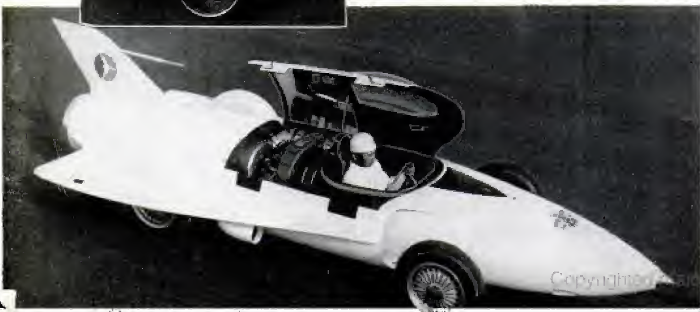
Above, expanding gas from burners spins turbine and the power goes through two-speed transmission to rear wheels. Below, engine is behind driver who sits in a tiny cockpit
